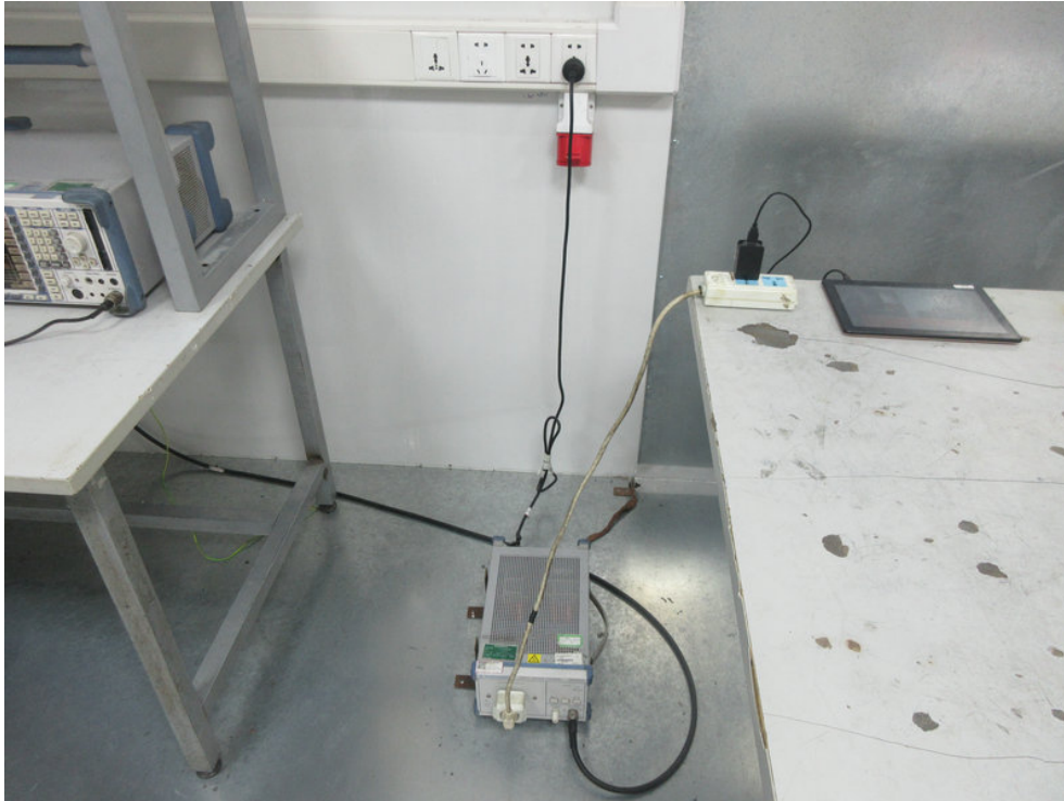
Photo of Conducted Emission Measurement
