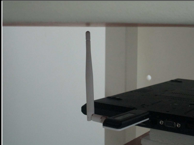
Test Position 11: USB Horizontal Down Tip of Antenna With 0.5 cm Gap (Antenna in Vertical 90 degree)
