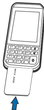
Figure 5 Inserting a Smart Card
