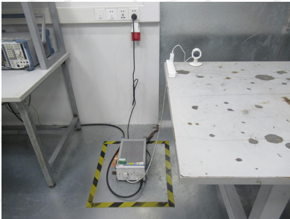
Photo of Power Line Conducted Emission Test
