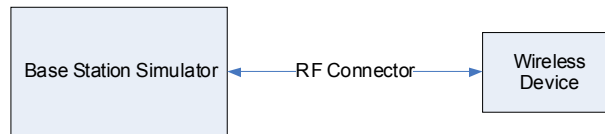
Figure 9-2 Power Measurement Setup
