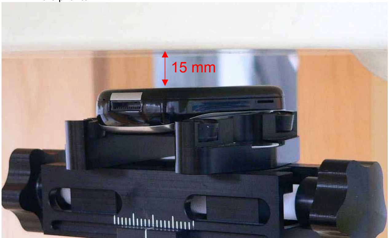
Fig. 33: Body worn configuration, GSM with headset, antenna towards the phantom
