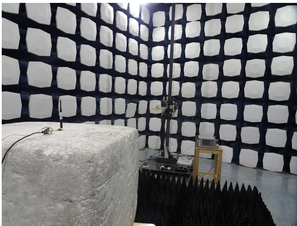
Picture 1 Radiated Emission Test Setup
