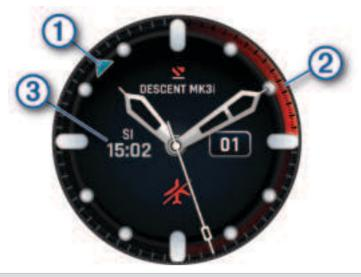
Alternate time zone pointer. References the 24-hour time markings on the watch (Adding Alternate Time Zones, page 4).
