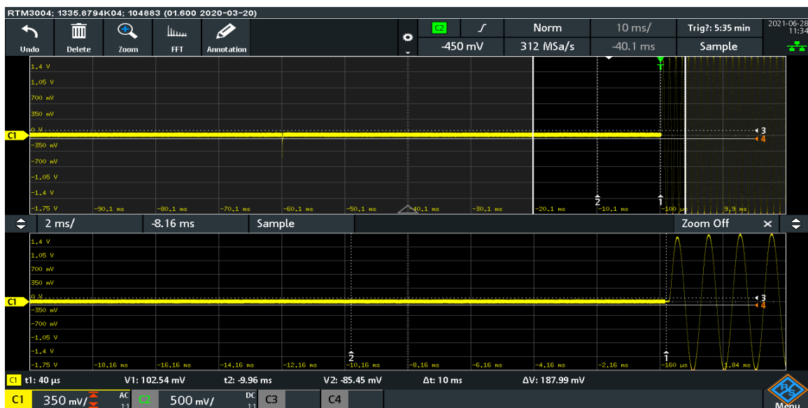
Plot 7.6.4 Transient frequency during power OFF test results at mid carrier frequency
