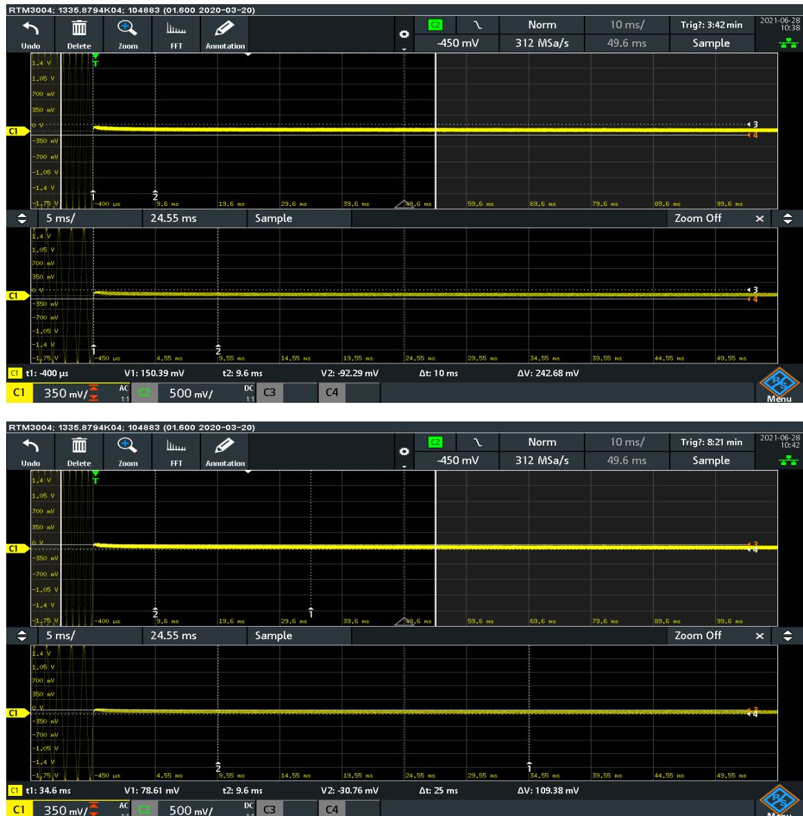
Plot 7.6.3 Transient frequency during power ON test results at mid carrier frequency
