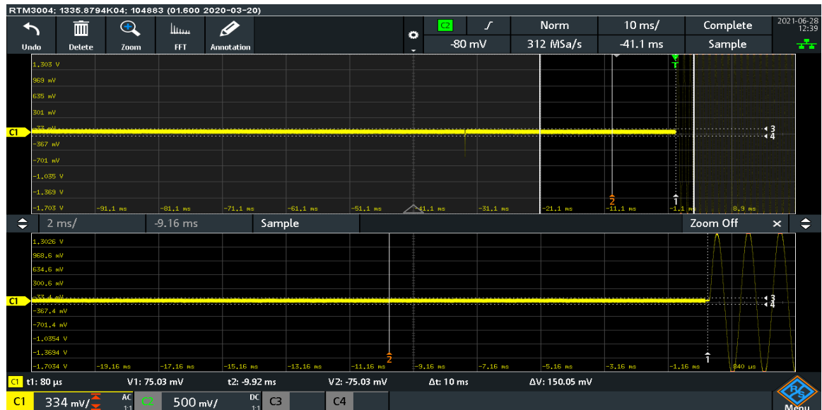
Plot 7.6.6 Transient frequency during power OFF test results at high carrier frequency
