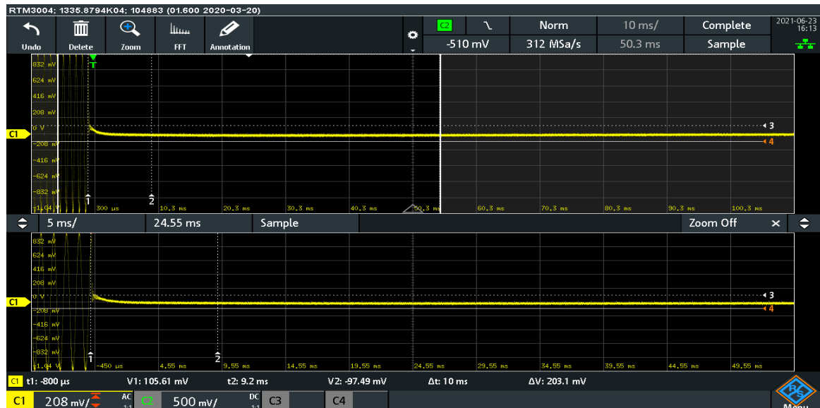
Plot 7.6.5 Transient frequency during power ON test results at high carrier frequency
