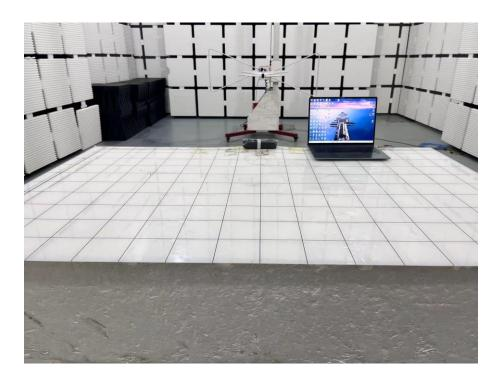
Set-up for Radiated Spurious Emission, Above 1GHz
