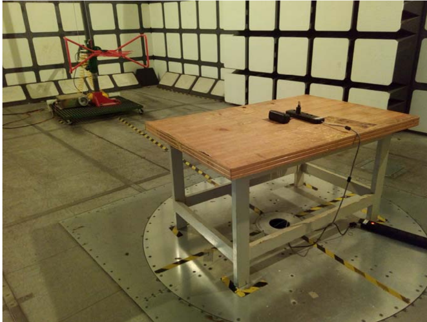
Radiated Emissions View (Below 1 GHz)
