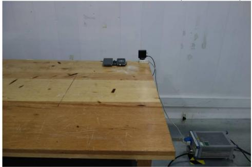
1.2 Radiated Emissions (9kHz-30MHz) Test Setup
