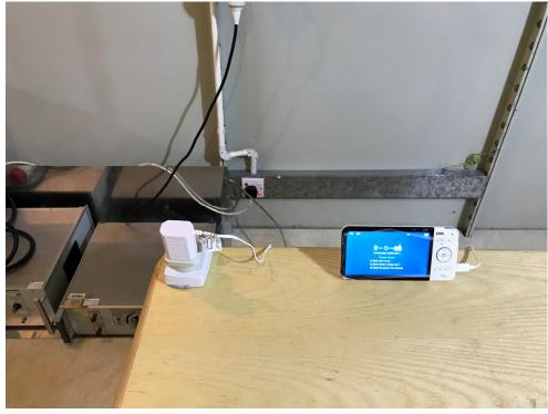
Radiated Emissions (30MHz-1GHz) Test Setup
