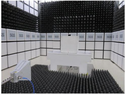
Conducted RF Output Power Test Setup
