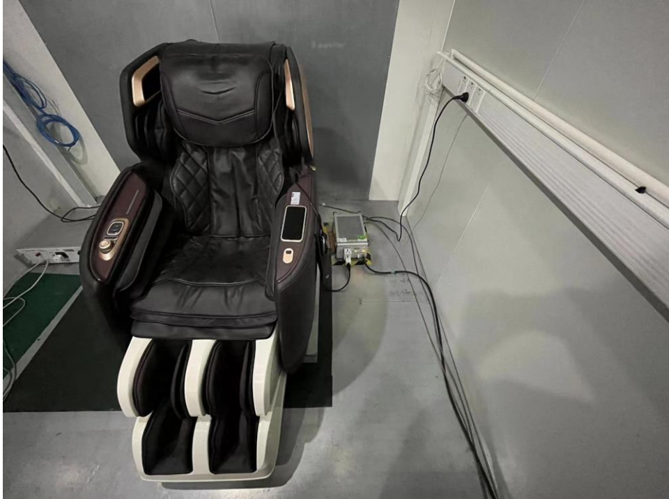
Conducted Emissions Test setup
