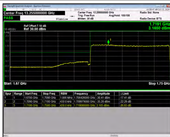
n66 SCS=15kHz DFT_16QAM BW=40MHz LowChannel=346000 RB=216@0
