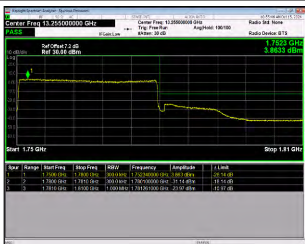
n66 SCS=15kHz DFT_QPSK BW=30MHz HighChannel=353000 RB=160@0
