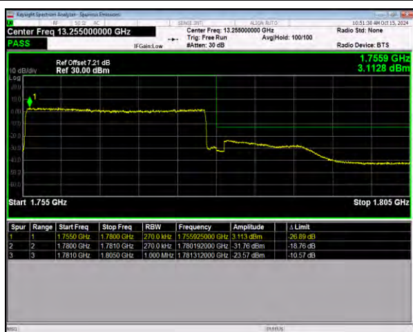
n66 SCS=15kHz DFT_64QAM BW=25MHz HighChannel=353500 RB=128@0
