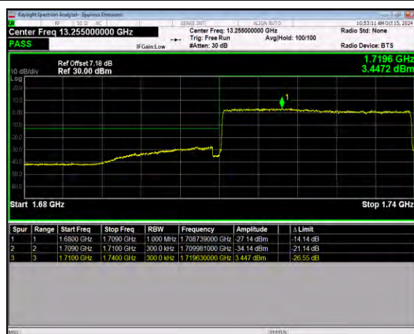
n66 SCS=15kHz DFT_QPSK BW=30MHz LowChannel=345000 RB=160@0
