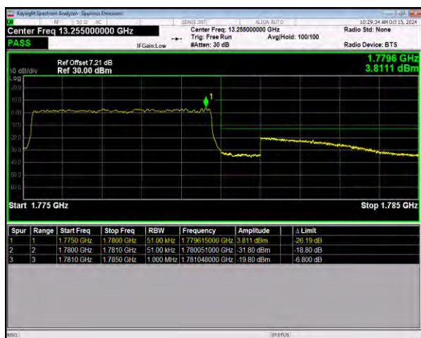
n66 SCS=15kHz DFT_16QAM BW=5MHz HighChannel=355500 RB=25@0
