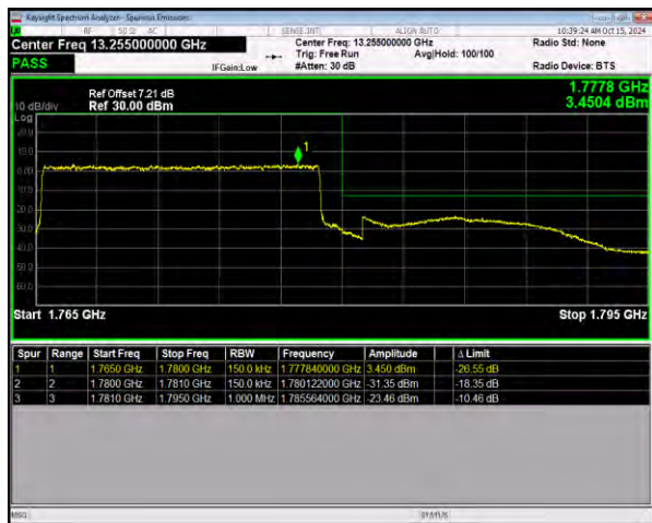
n66 SCS=15kHz DFT_BPSK BW=15MHz HighChannel=354500 RB=75@0
