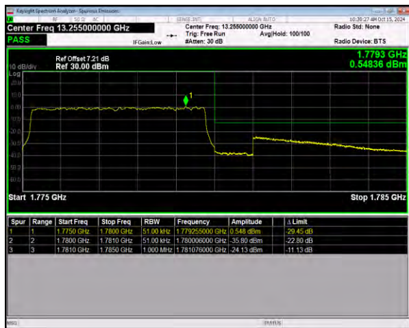
n66 SCS=15kHz DFT_256QAM BW=5MHz HighChannel=355500 RB=25@0
