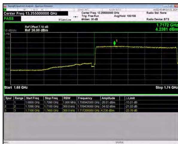
n66 SCS=15kHz DFT_BPSK BW=30MHz LowChannel=345000 RB=160@0
