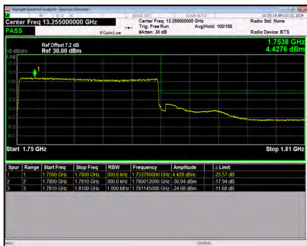
n66 SCS=15kHz DFT_BPSK BW=30MHz HighChannel=353000 RB=160@0
