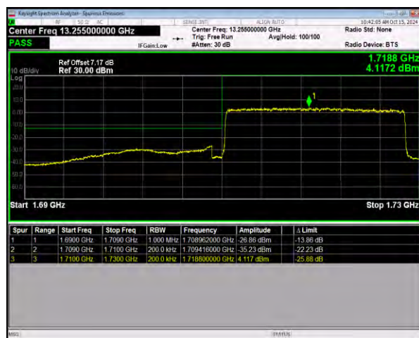
n66 SCS=15kHz DFT_BPSK BW=20MHz LowChannel=344000 RB=100@0
