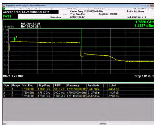
n66 SCS=15kHz CP_QPSK BW=30MHz HighChannel=353000
