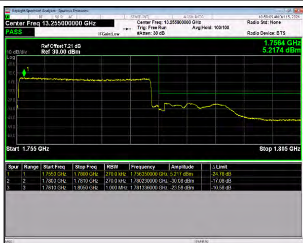
n66 SCS=15kHz DFT_BPSK BW=25MHz HighChannel=353500
