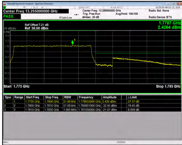
n66 SCS=15kHz DFT_64QAM BW=5MHz HighChannel=355500 RB=25@0
