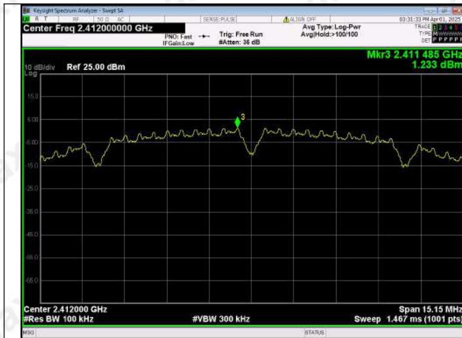
In-Band Reference Level IEEE 802.11b_Channel 1_20MHz
