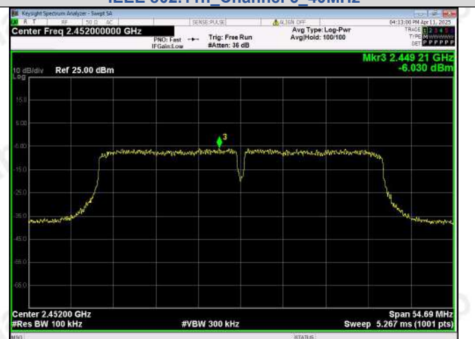
In-Band Reference Level IEEE 802.11n_Channel 9_40MHz
