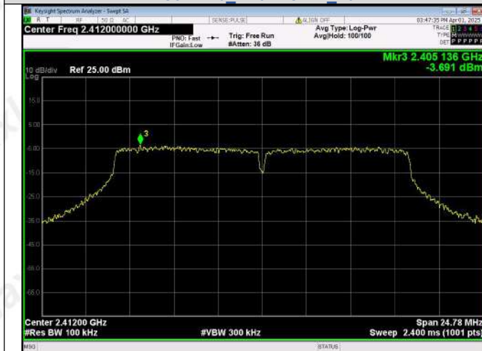
In-Band Reference Level IEEE 802.11g Channel 1 20MHz
