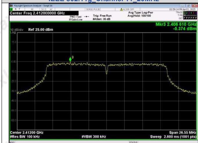
In-Band Reference Level IEEE 802.11n_Channel 1_20MHz
