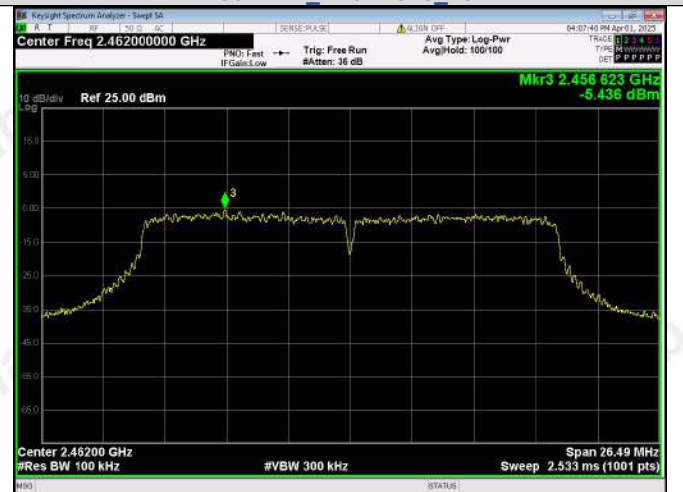
In-Band Reference Level IEEE 802.11n_Channel 11_20MHz
