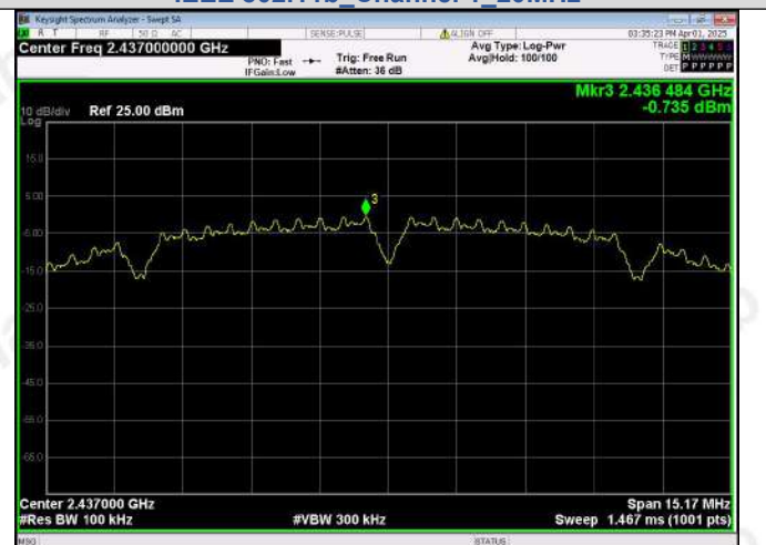
In-Band Reference Level IEEE 802.11b_Channel 6_20MHz
