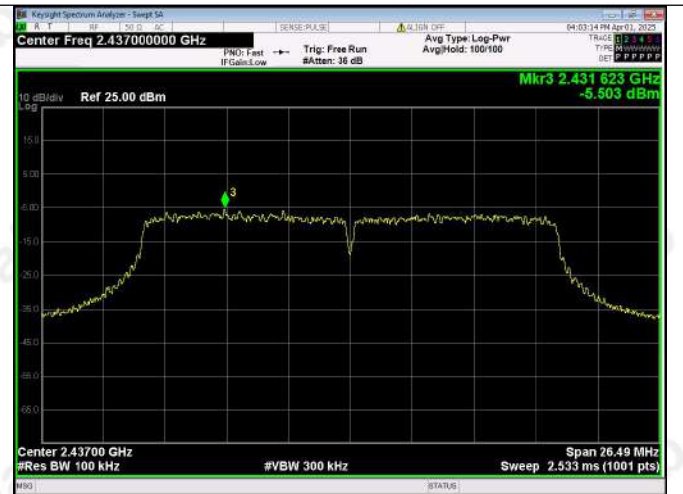
In-Band Reference Level IEEE 802.11n_Channel 6_20MHz
