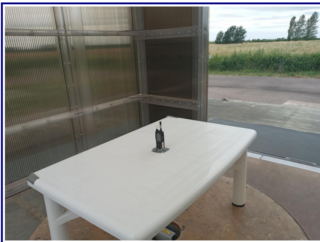
Photo 2: Radiated Emissions : Helical Antenna
