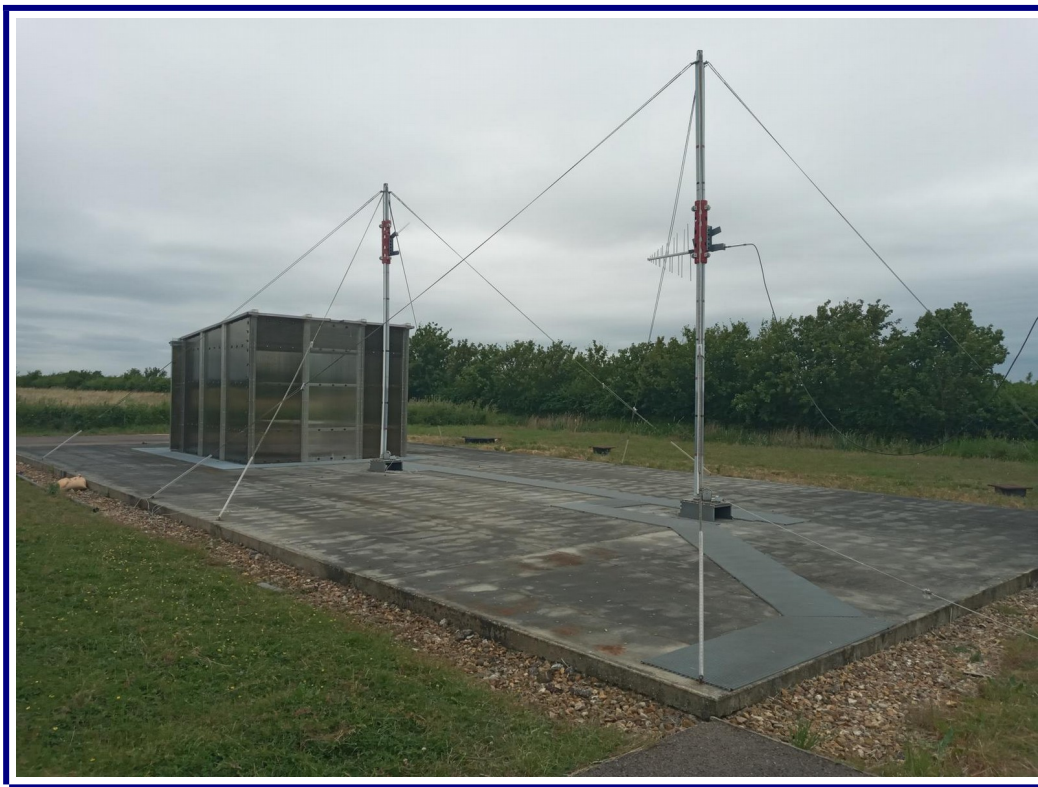
Photo 1: Radiated Emissions : Polar plot measurement setup
