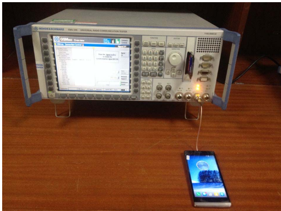
Photograph –2G&3G Conducted Test Setup
