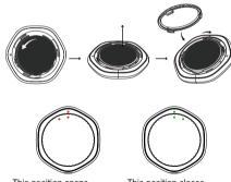
This position opens the battery compartment
