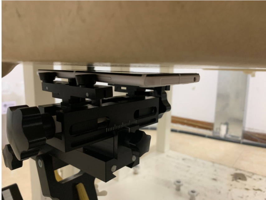
Body worn _ Front (Test distance: 5mm, Thickness of DUT: 9mm)
