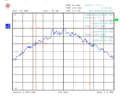
Modulation Type: GFSK (Channel 00) :
