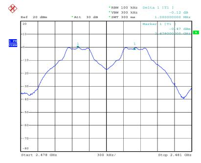
Modulation Type: GFSK (Channel 78) :
