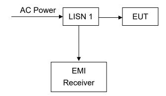
The EUT are connected to the main power through a line impedance stabilization network (LISN). This provides a 50 ohm/50 uH coupling impedance for the measuring equipment. The peripheral devices are also connected to the main power through a LISN that provides a 50 ohm/50 uH coupling impedance with 50 ohm termination.
