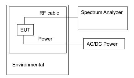
Note1:The frequency stability is measured with the temperature variation range of -20°C to +45°C, and voltage supply variation range of 85% to 115% of nominal DC supply voltage.
