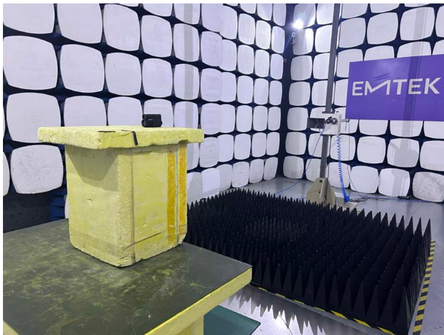
Spurious Emission Test Setup (Above 1GHz)
