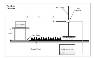
The radiated emission tests were performed in the 3 meters chamber test site, using the setup accordance
