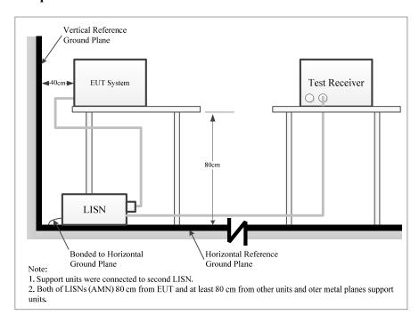
The measurement procedure of test setup is according with ANSI C63.4-2014. The related limit was specified in FCC Part 15.107 Class B limits.
