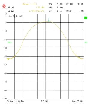
Raymarine EUT: Smart Controller. Peak Power FCC P15.247 Comment A: 46813 Bottom Channel Date: 24.NOV.2004 14:05:03
