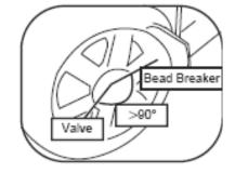
2.2 Firmly fix the wheel on the turntable clamps. (If the mounting head of the tyre changer is positioned at 12 o'clock, then the valves stem should be at the 11 o'clock position.) Apply lubricant to both tyre bead and rim, and then remove the upper tyre bead.
