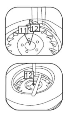
2.4 Final inspection: Visually inspect the rim, valve stem and electronic module to ensure no damage has occurred.
