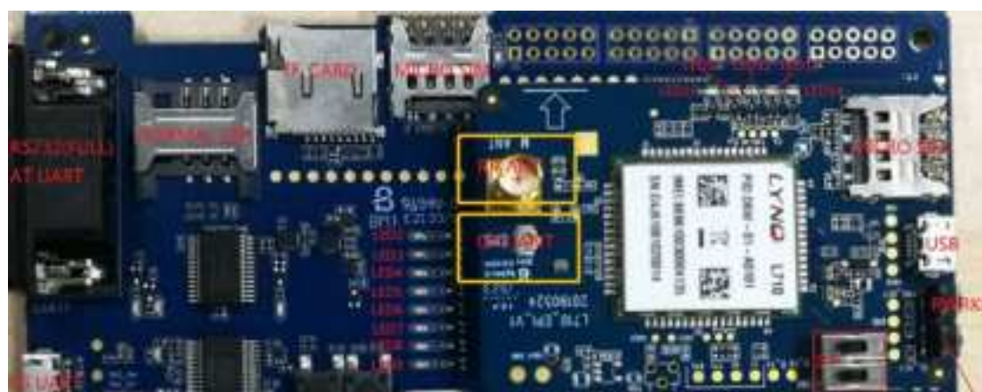
Figure5-7: Function module load plate and antenna interface
