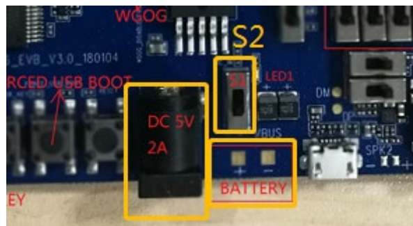
Figure 3-1: L710HG development board power in Status (orange Power LED Light up)
