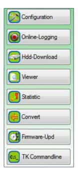
Function Tool Configuration Customise the N4000+ behaviour **Online-Logging** Start and stop logging Hdd-Download Download measurements from the N4000+ storage medium Viewer Evaluate measurements Evaluate bus statistics Statistic Convert Convert log data to other formats Update firmware Firmware-Update **TK Commandline** Command line access to the XORAYAToolkit
