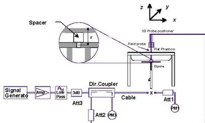
**Figure 12.1 Dipole Validation 1**
