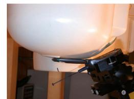
**Figure 14.1 Right Head SAR Test Setup
