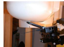
**Figure 14.6 Right Head SAR Test Setup
