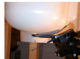
**Figure 14.5 Right Head SAR Test Setup
