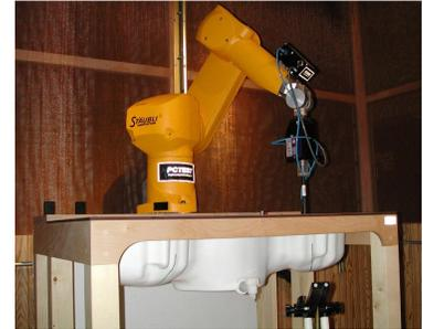
**Figure 6.1** DASY4 Test System
