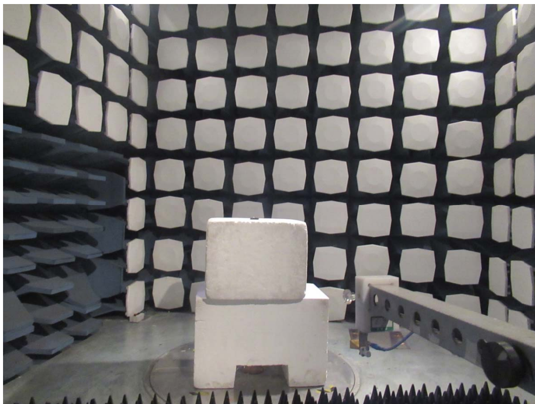
Picture 1: Radiated Spurious Emissions Test setup
