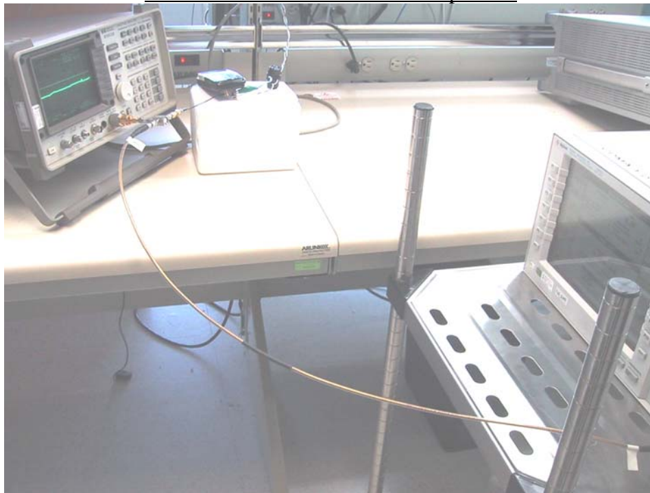
RF Conducted Emission Test-Setup Photo
