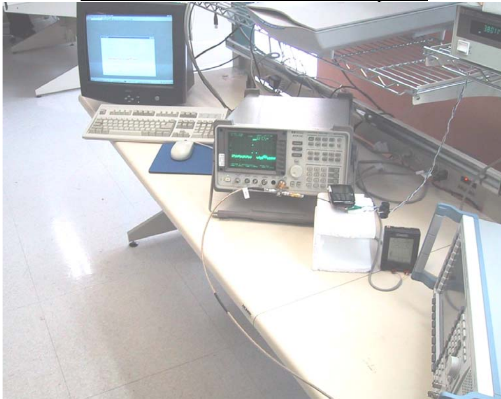
RF Conducted Bluetooth Emission Test-Setup Photo
