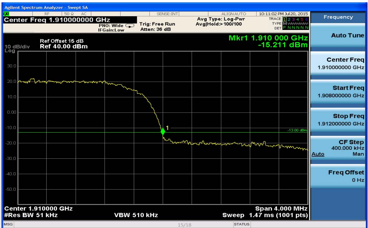
Fig.10 WCDMA Band II-CH9538Band Edge Compliance
