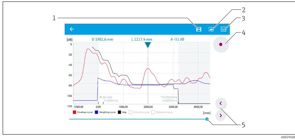
8 Envelope curve display (example) in SmartBlue; Android view
