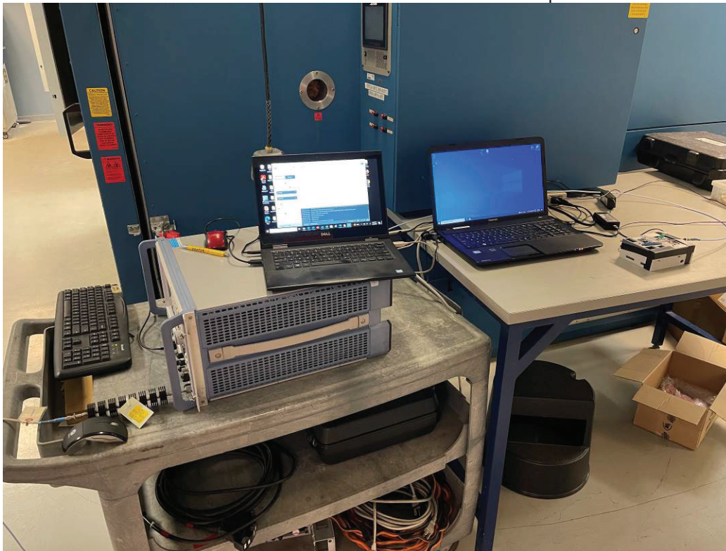
Antenna Port Conducted Emission Test Setup
