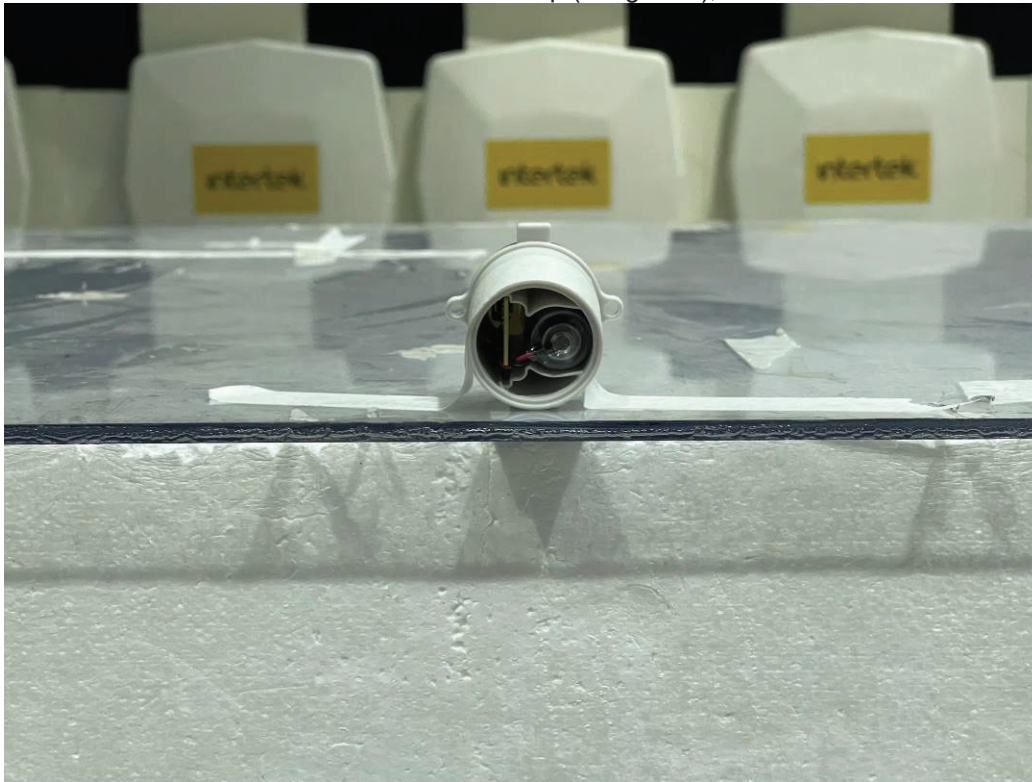
Radiated Emission Test Setup (Long Side), 1-13 GHz
