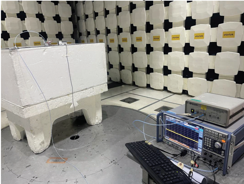
Radiated Emission Manual Testing Setup, 18-25 GHz
