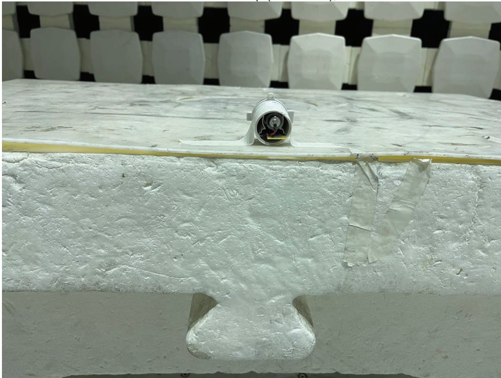
Radiated Emission Test Setup (Back Side), 30-1000 MHz
