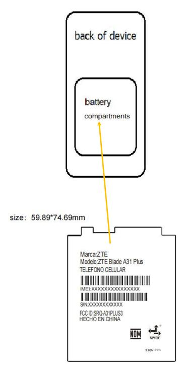
The label is on the device which is under the battery.
