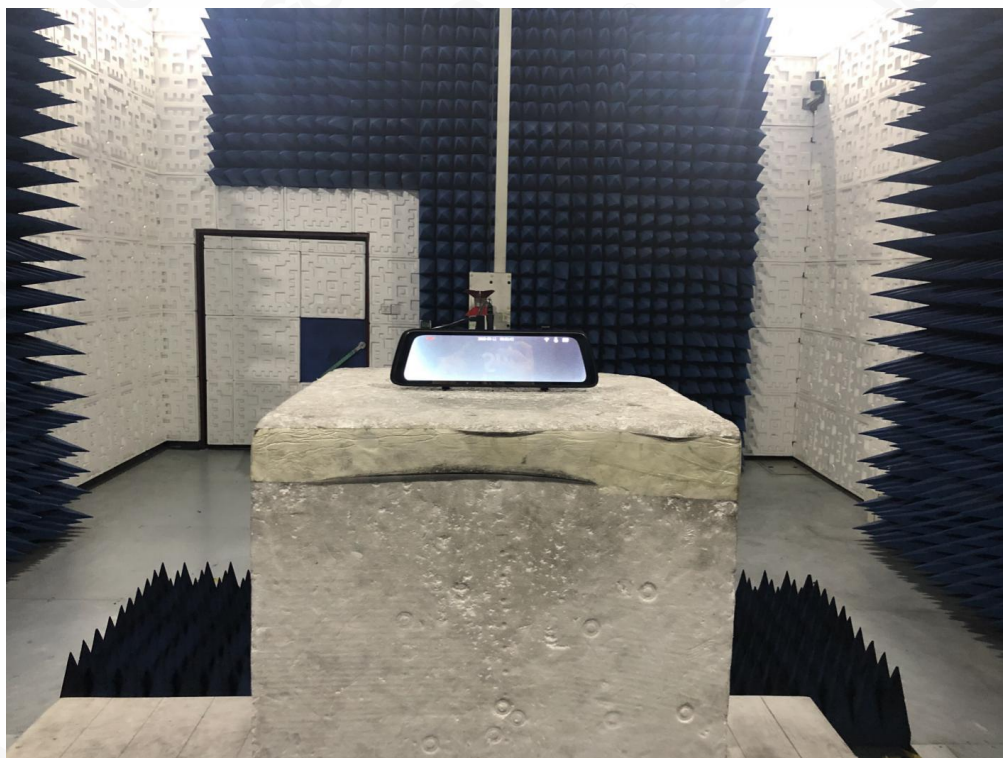
FCC RADIATED EMISSION TEST SETUP ABOVE 1GHZ
