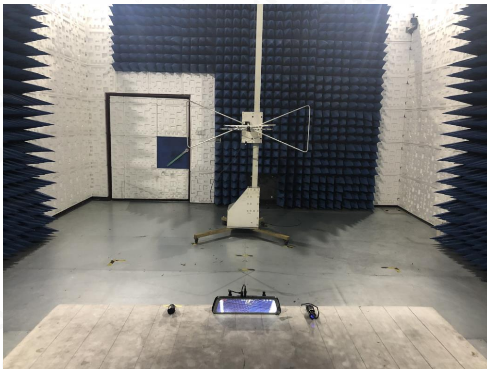
FCC RADIATED EMISSION TEST SETUP ABOVE 1GHZ
