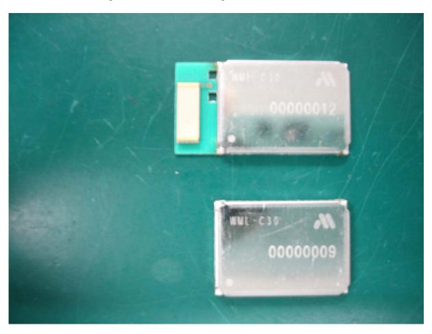
Bottom view. Module with integral antenna and without
