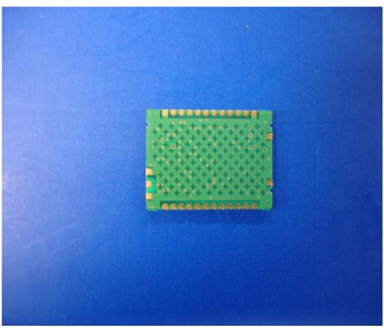
Photo without shielded case. Module with integral antenna and without
