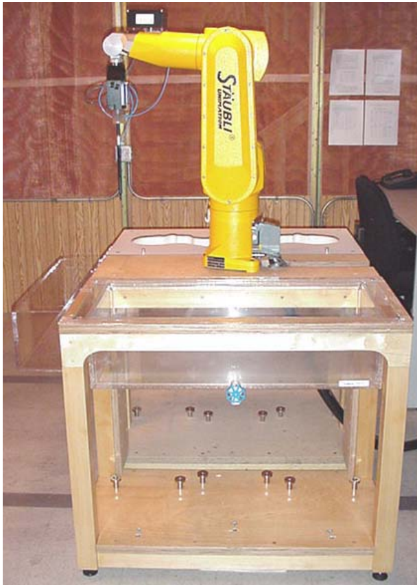
DASY4 SAR Measurement System with validation phantom
