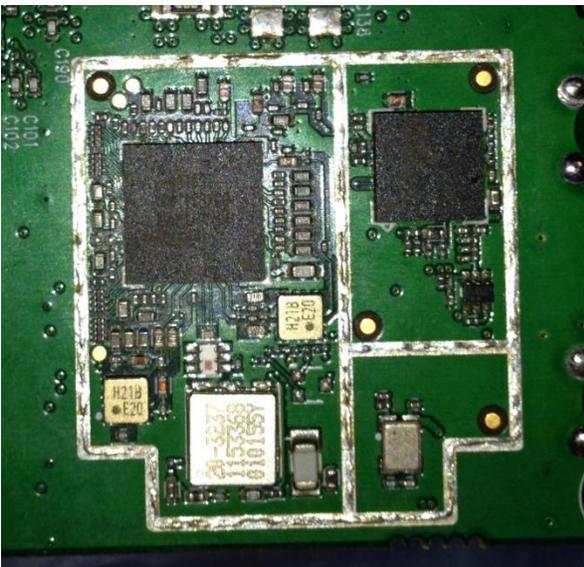
Figure 8 - Satellite communication radio, lower portion, shield removed
