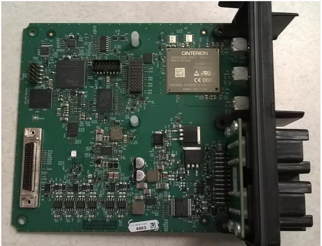
Figure 9 - Main board with daughterboard removed
