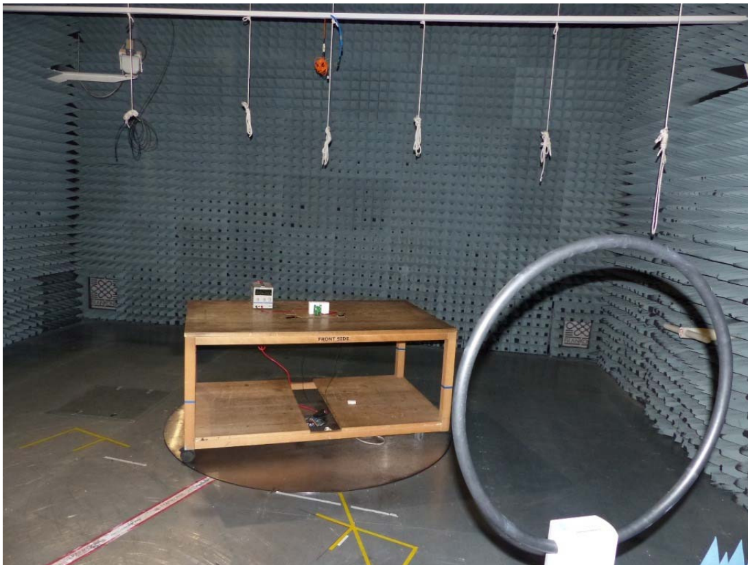
Photo 5: Test setup for radiated measurements (below 30 MHz)
