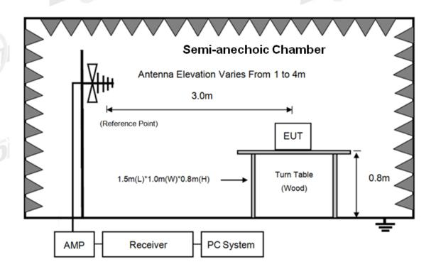
Semi-Anechoic 3m Chamber
