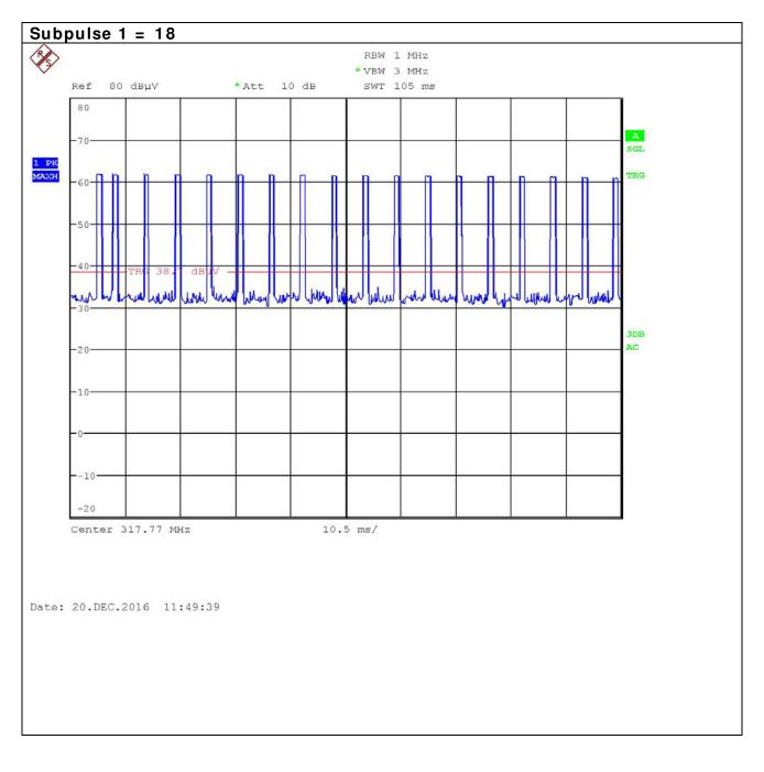
Test Data: 100 ms Number of Pulses Plot
