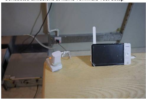
Radiated Emissions (30MHz-1GHz) Test Setup
