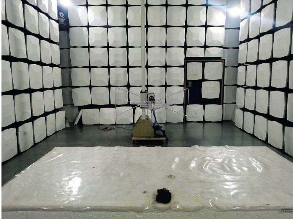
Radiated Emission Test Setup:
