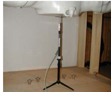
Figure 12.1 Dipole Validation Test Setup
