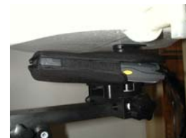
Figure 14.1 Body SAR Test Setup -- w/ Holster --
