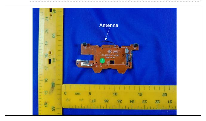
Details of: PCB view for remote controller
