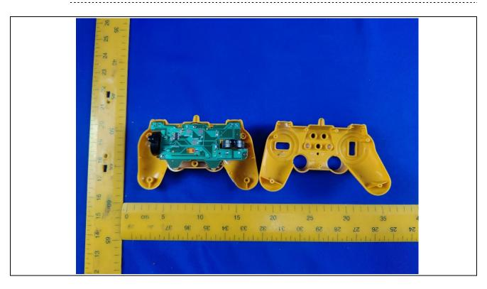
Details of: PCB view for remote controller
