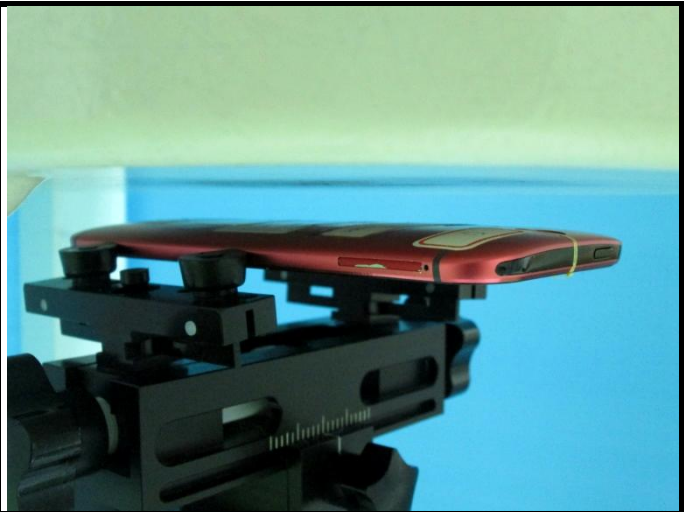
Rear Face of EUT with 1.0 cm Gap
