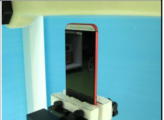
Bottom Side of EUT with 1.0 cm Gap
