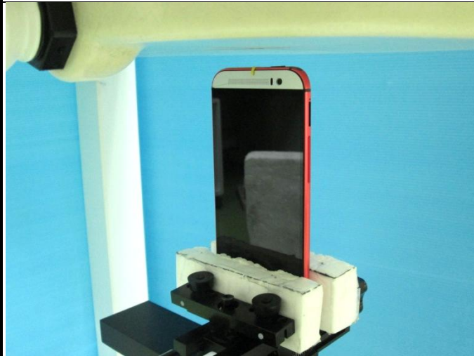
Top Side of EUT with 1.0 cm Gap
