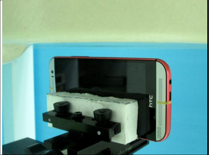
Right Side of EUT with 1.0 cm Gap
