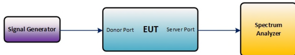
Figure 5 – Intermodulation product instrumentation test setup
