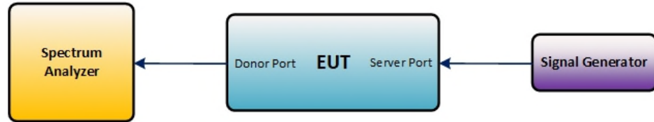
Figure 3 – Downlink test configuration in EUT test mode
