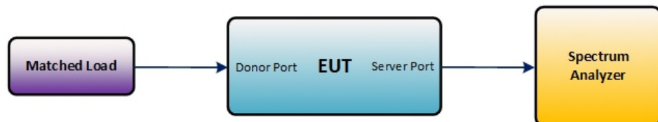
Figure 6 – Maximum downlink noise limit test configuration
