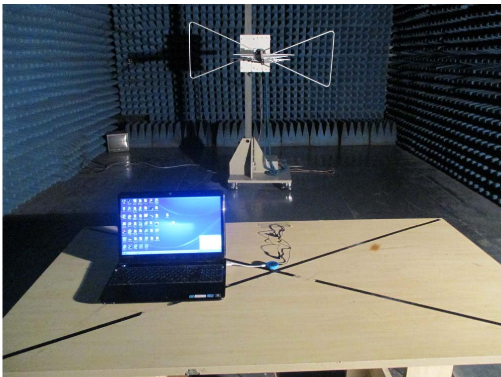
FCC RADIATED EMISSION TEST SETUP
