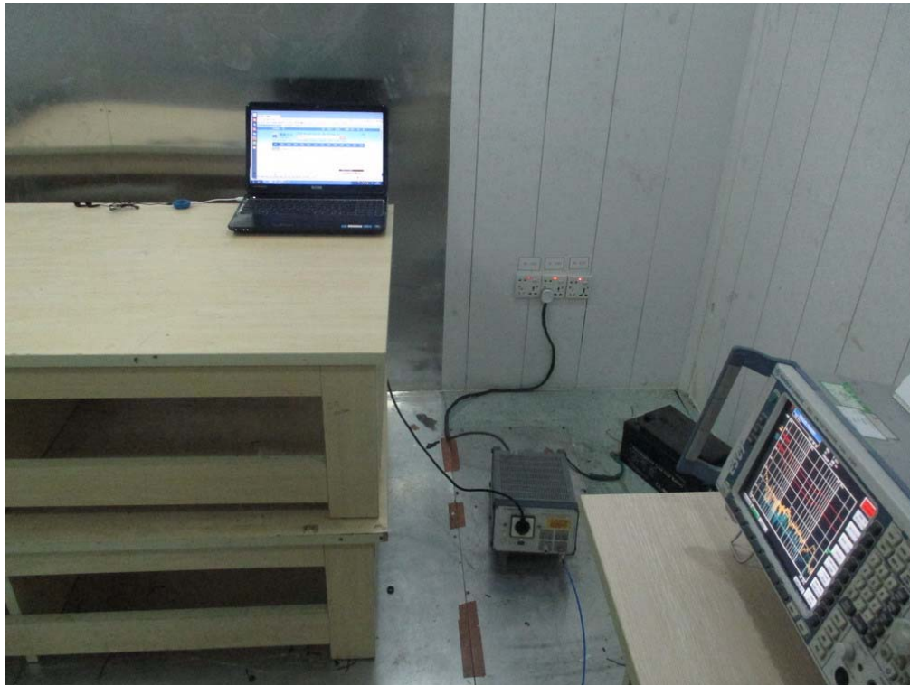
FCC RADIATED EMISSION TEST SETUP
