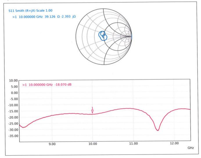
Measurement Report for 5G Verification Source 10 GHz, UID 0 -, Channel 10000.0 (10000.0 MHz)
