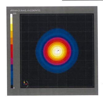
Measurement Report for 5G Verification Source 10 GHz, UID 0 -, Channel 10000.0 (10000.0 MHz)
